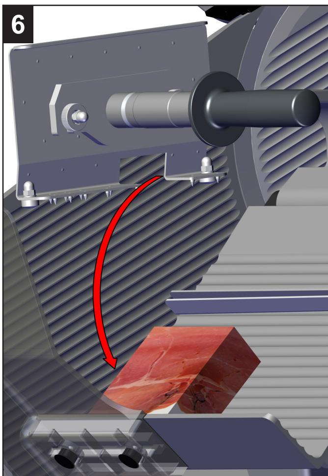
Locate the gripper arm onto the product
