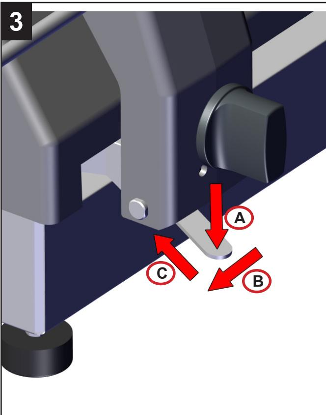
Press the "A" lever, push in "B" direction and stop in "C" position
