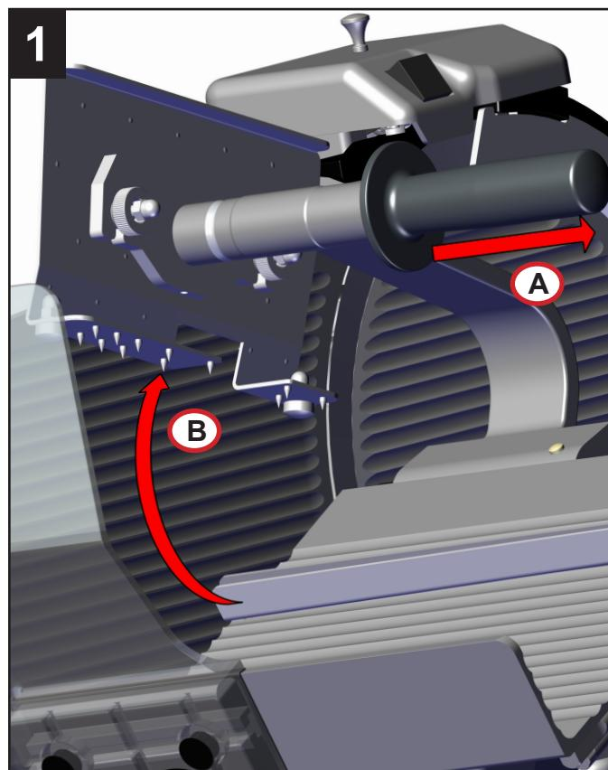
Lift the gripper arm (A), (B)
