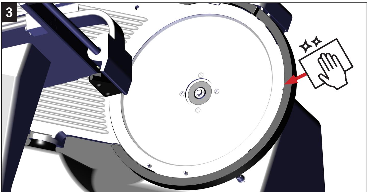
Carefully insert the doth betwen the knife and the knife ring guard. While holding the cloth between the knife and the ring guard, work it along the entire backside of the knife. Repeat this procedure as necessary . A nylon brush could also be used.
