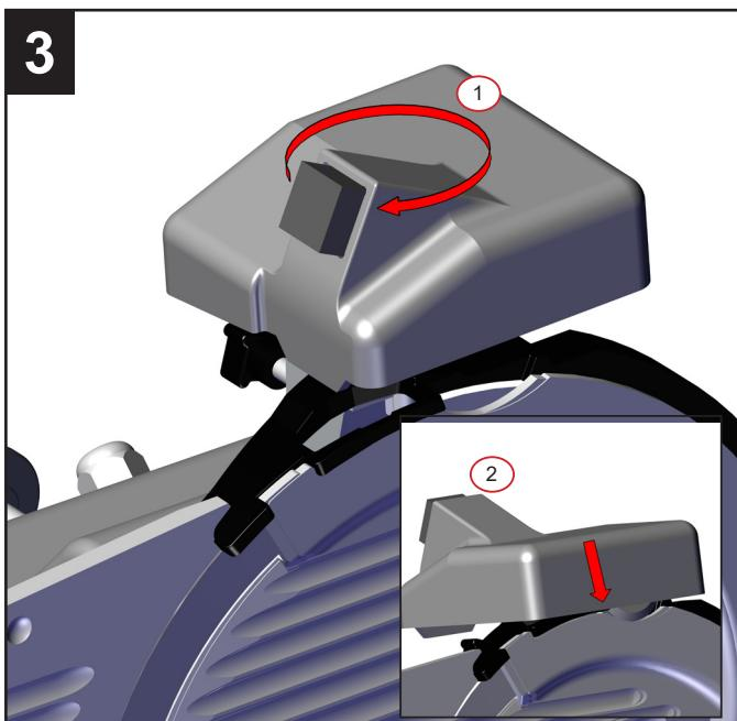
C) Turn the sharpener by 180° and insert the wheels on the slicer blade.
