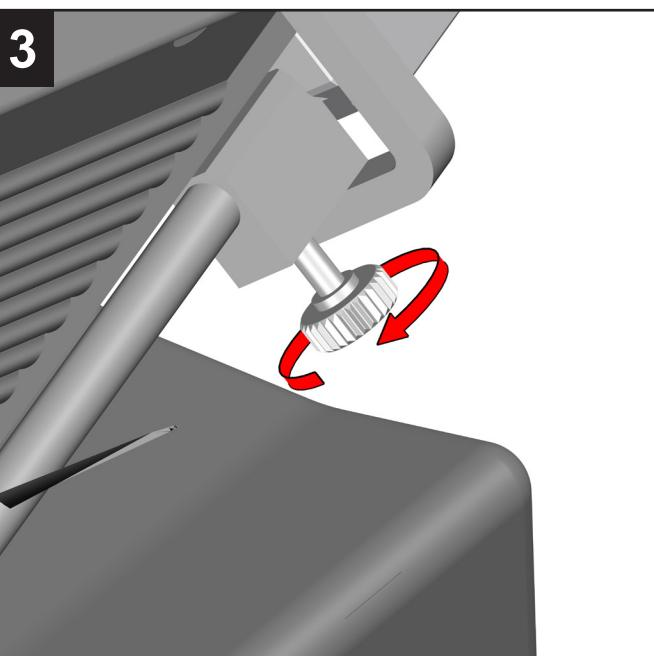
Unscrew the fence retaining knob and slide the fence in to the outer position
