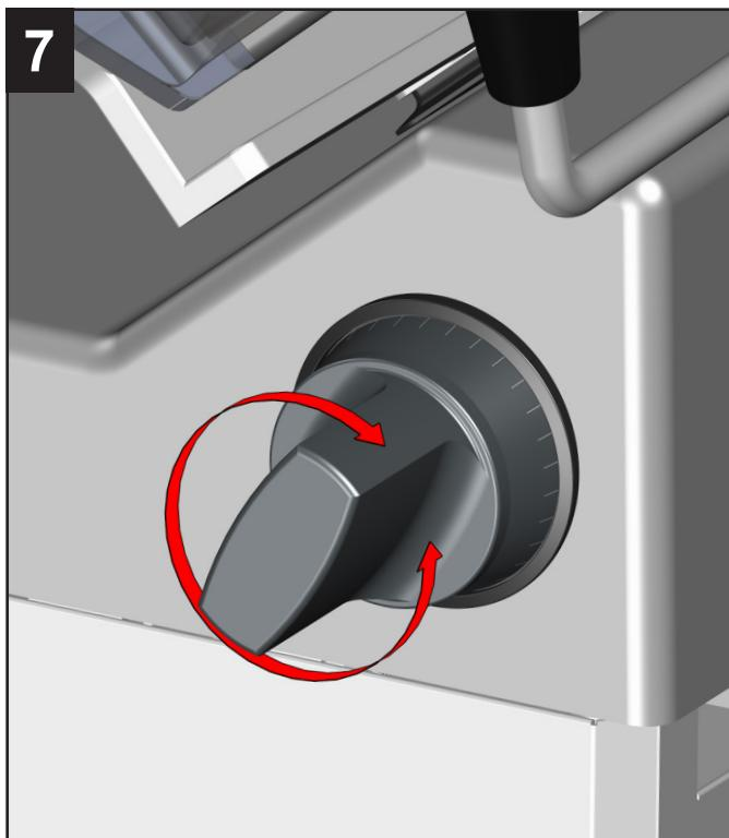
Select the thickness of the product to be sliced using the portion thickness control knob
