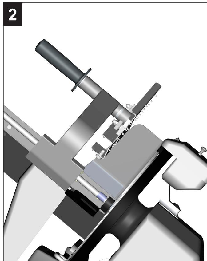
Lock the gripper arm into the rest position
